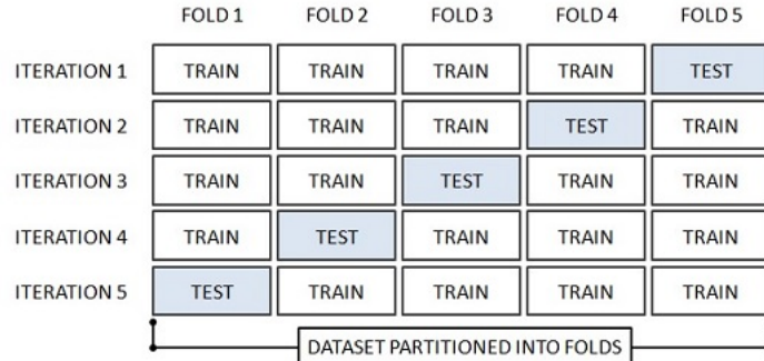
Figure 2.15: Example of 5-fold cross validation. Test set is selected differently in each iteration. Models are trained on the remaining folds.
