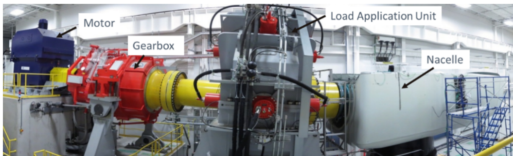
Figure 1.1: Clemson University's 7.5 MW Test Bench
