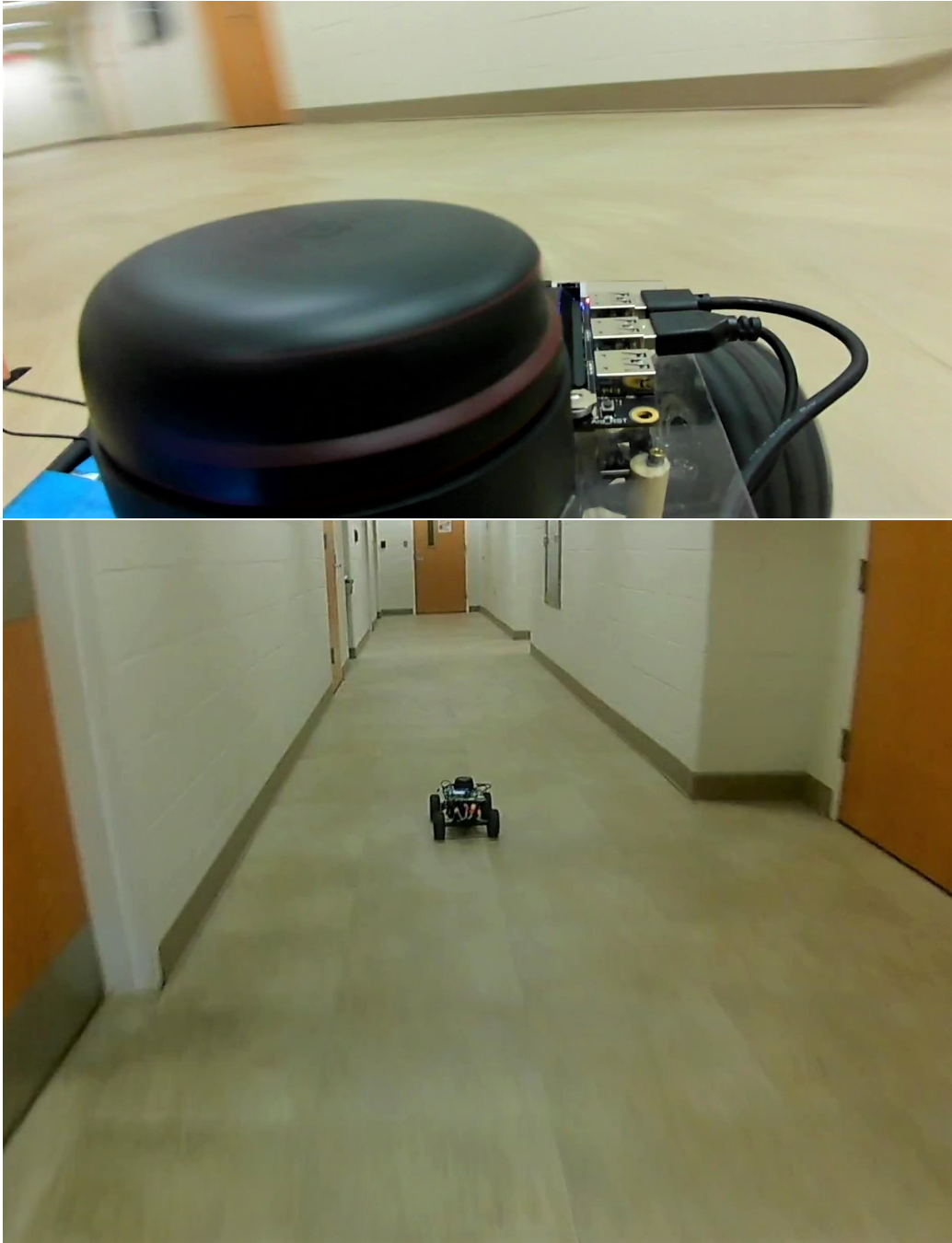
Figure 5: Onboard testing of high speed navigation of 1/12 scaled ackermann steering robot
