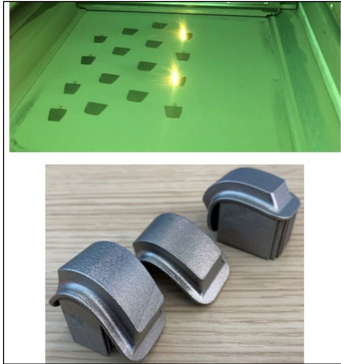
Figure 7.1: Parts during print and after removal from build-plate.
