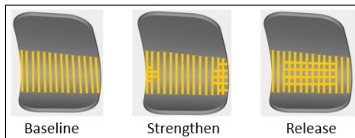
Figure 2.4: The three strategies viewed from the bottom showing the differing support structures in yellow.
