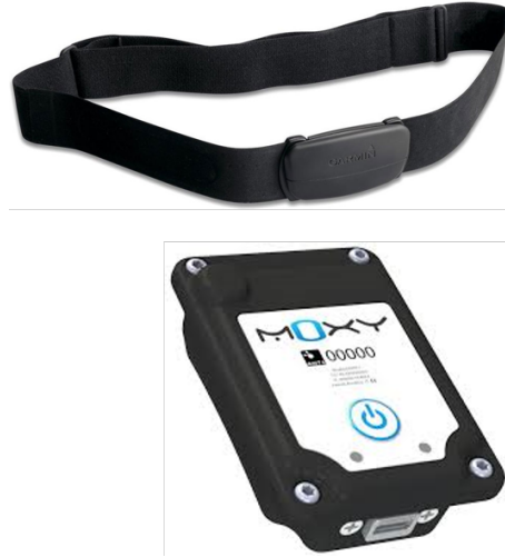
Figure 2.2: The Garmin heart rate (top), and Moxy muscle oxygenation (bottom) sensors used in the experiments.
