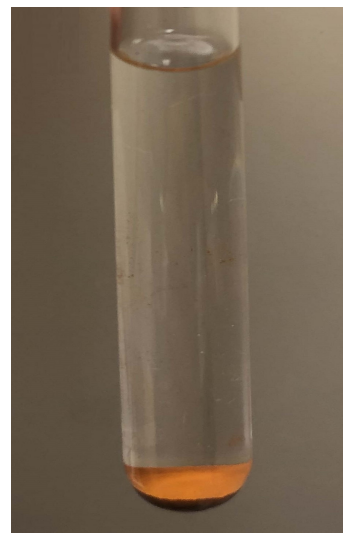
Figure B.15: 0.5 wt.% of \text{Fe}_2\text{O}_3 with 1.0 wt.% SDS.
