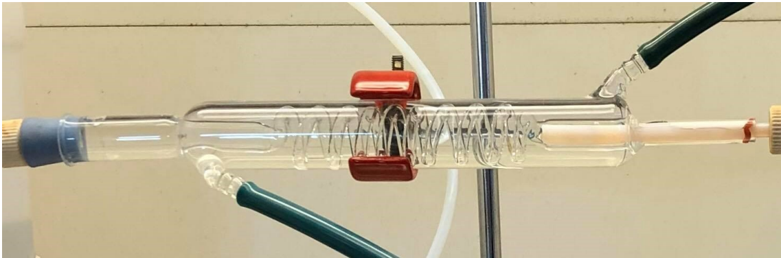
Figure 3.3: Heat exchanger used in the experimental apparatus. The left and right assembly configuration between the tube and the heat exchanger are visualized.
