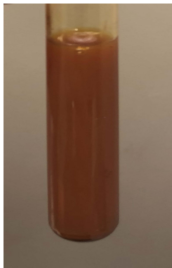
Figure B.14: 0.5 wt.% of \text{Fe}_2\text{O}_3 with 1.0 wt.% PVP.
