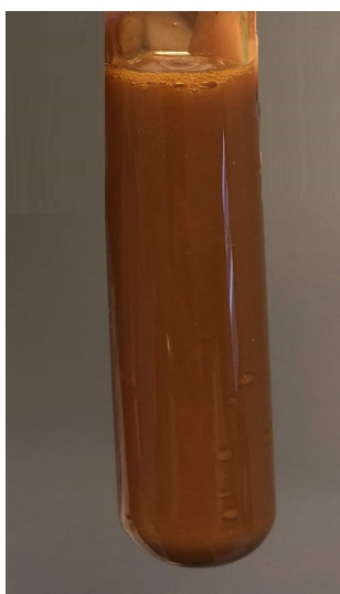
Figure 3.7: 1.0 wt.% of \text{Fe}_2\text{O}_3 with 1.0 wt.% PVP, after sonification.
