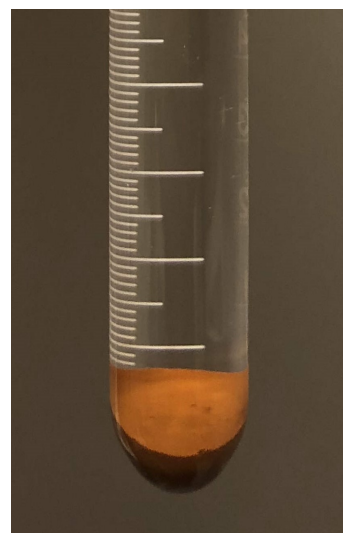
Figure B.21: 1.5 wt.% of \text{Fe}_2\text{O}_3 with 1.0 wt.% SDS.
