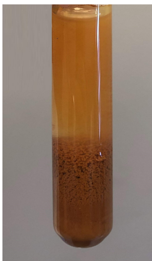
Figure 3.12: 1.0 wt.% of \text{Fe}_2\text{O}_3 without dispersant and \text{pH}=2.2 , after sonification.
