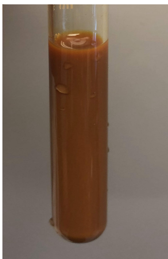
Figure B.7: 1.5 wt.% of \text{Fe}_2\text{O}_3 without dispersant.
