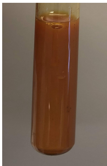
Figure B.2: 0.5 wt.% of \text{Fe}_2\text{O}_3 with 1.0 wt.% PVP.
