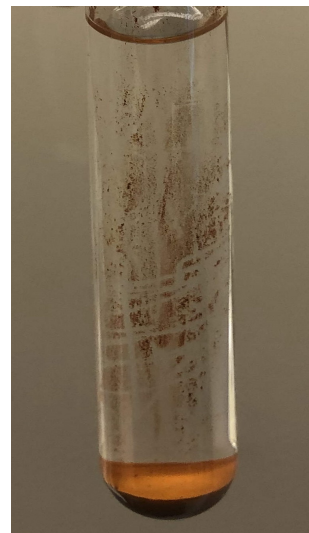
Figure 3.11: 1.0 wt.% of \text{Fe}_2\text{O}_3 with 1.0 wt.% SDS, 24 hours after sonification.
