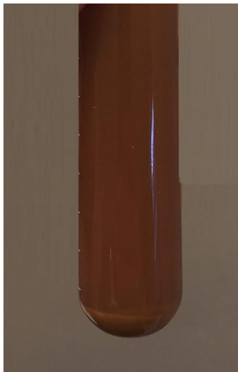
Figure B.17: 1.0 wt.% of \text{Fe}_2\text{O}_3 with 1.0 wt.% PVP.
