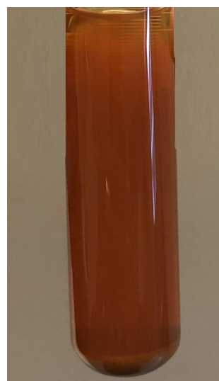
Figure 3.17: 1.0 wt.% of \text{Fe}_2\text{O}_3 with \text{pH} = 10.1 , 24 hours after sonification.
