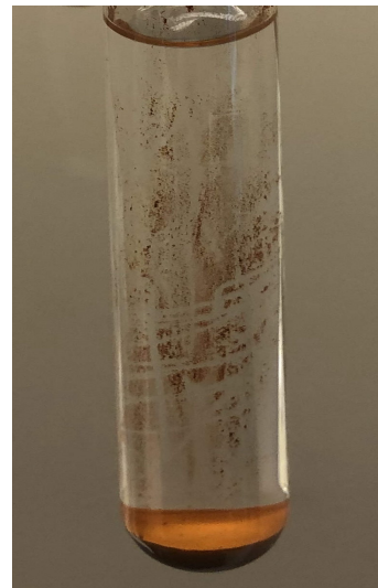
Figure B.18: 1.0 wt.% of \text{Fe}_2\text{O}_3 with 1.0 wt.% SDS.
