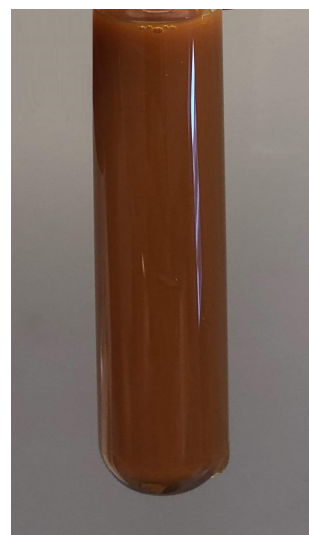
Figure 3.14: 1.0 wt.% of \text{Fe}_2\text{O}_3 with \text{pH} = 10.1 , after sonification.
