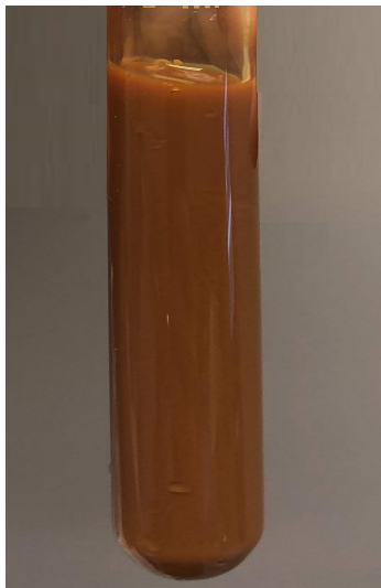
Figure B.4: 1.0 wt.% of \text{Fe}_2\text{O}_3 without dispersant.
