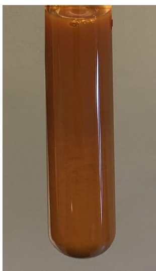
Figure 3.16: 1.0 wt.% of \text{Fe}_2\text{O}_3 with \text{pH} = 7.3 , 24 hours after sonification.
