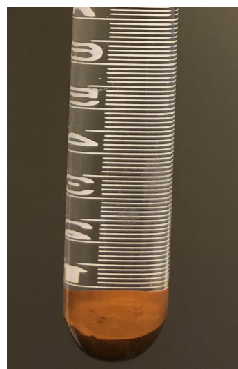
Figure B.24: 2.0 wt.% of \text{Fe}_2\text{O}_3 with 1.0 wt.% SDS.
