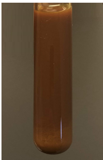
Figure B.19: 1.5 wt.% of \text{Fe}_2\text{O}_3 without dispersant.
