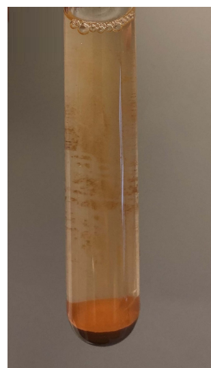
Figure 3.8: 1.0 wt.% of \text{Fe}_2\text{O}_3 with 1.0 wt.% SDS, after sonification.
