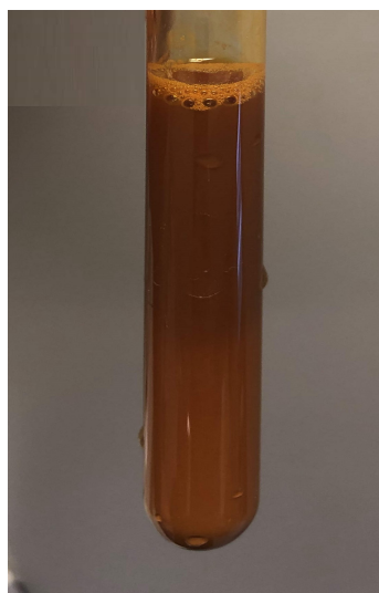
Figure B.11: 2.0 wt.% of \text{Fe}_2\text{O}_3 with 1.0 wt.% PVP.
