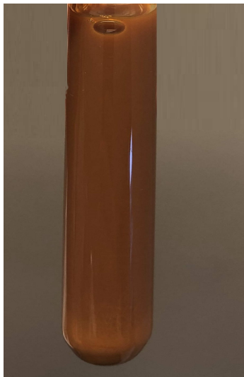
Figure B.16: 1.0 wt.% of \text{Fe}_2\text{O}_3 without dispersant.
