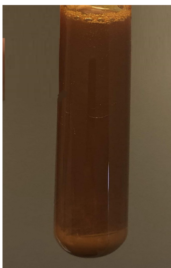
Figure B.23: 2.0 wt.% of \text{Fe}_2\text{O}_3 with 1.0 wt.% PVP.
