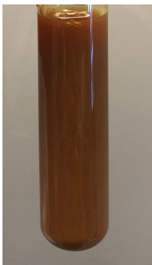
Figure 3.13: 1.0 wt.% of \text{Fe}_2\text{O}_3 with \text{pH} = 7.3 , after sonification.
