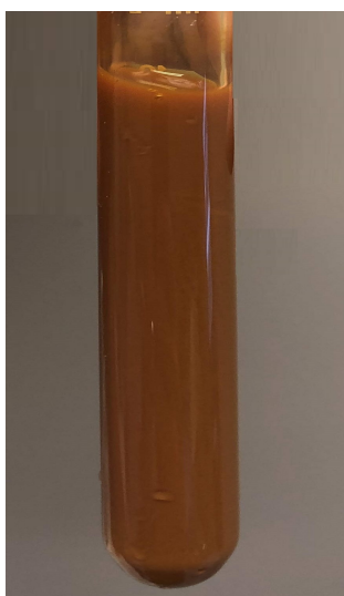
Figure 3.6: 1.0 wt.% of \text{Fe}_2\text{O}_3 without dispersant, after sonification.
