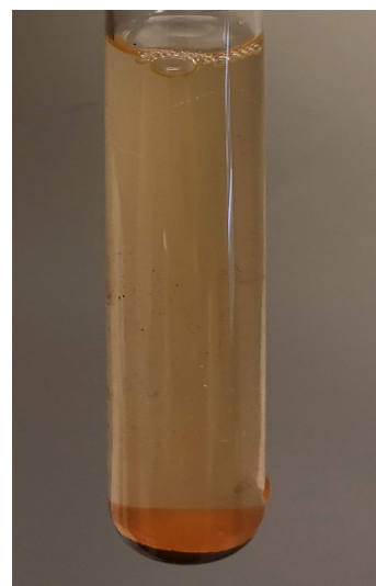
Figure B.3: 0.5 wt.% of \text{Fe}_2\text{O}_3 with 1.0 wt.% SDS.
