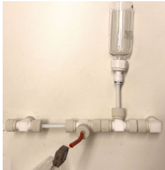
Figure 3.5: The assembly of temperature sensor T_2 and the expansion tank, with the apparatus in horizontal orientation.
