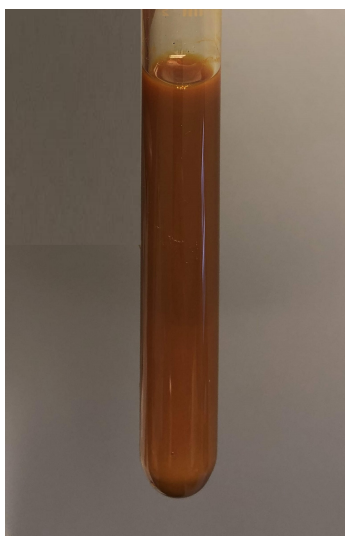
Figure B.10: 2.0 wt.% of \text{Fe}_2\text{O}_3 without dispersant.
