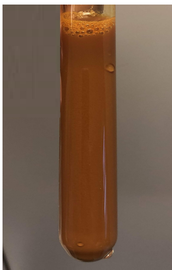
Figure B.8: 1.5 wt.% of \text{Fe}_2\text{O}_3 with 1.0 wt.% PVP.
