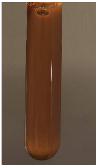
Figure 3.9: 1.0 wt.% of \text{Fe}_2\text{O}_3 without dispersant, 24 hours after sonification.
