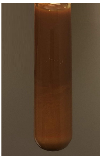
Figure B.22: 2.0 wt.% of \text{Fe}_2\text{O}_3 without dispersant.
