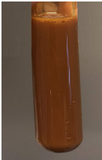
Figure B.5: 1.0 wt.% of \text{Fe}_2\text{O}_3 with 1.0 wt.% PVP.
