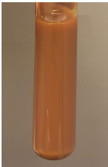
Figure B.13: 0.5 wt.% of \text{Fe}_2\text{O}_3 without dispersant.
