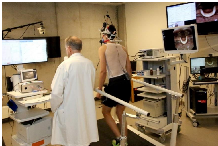
Figure 6: Set up for continuous laryngoscopy exercise-test (CLE-test), as described by Heimdal et al [3].
