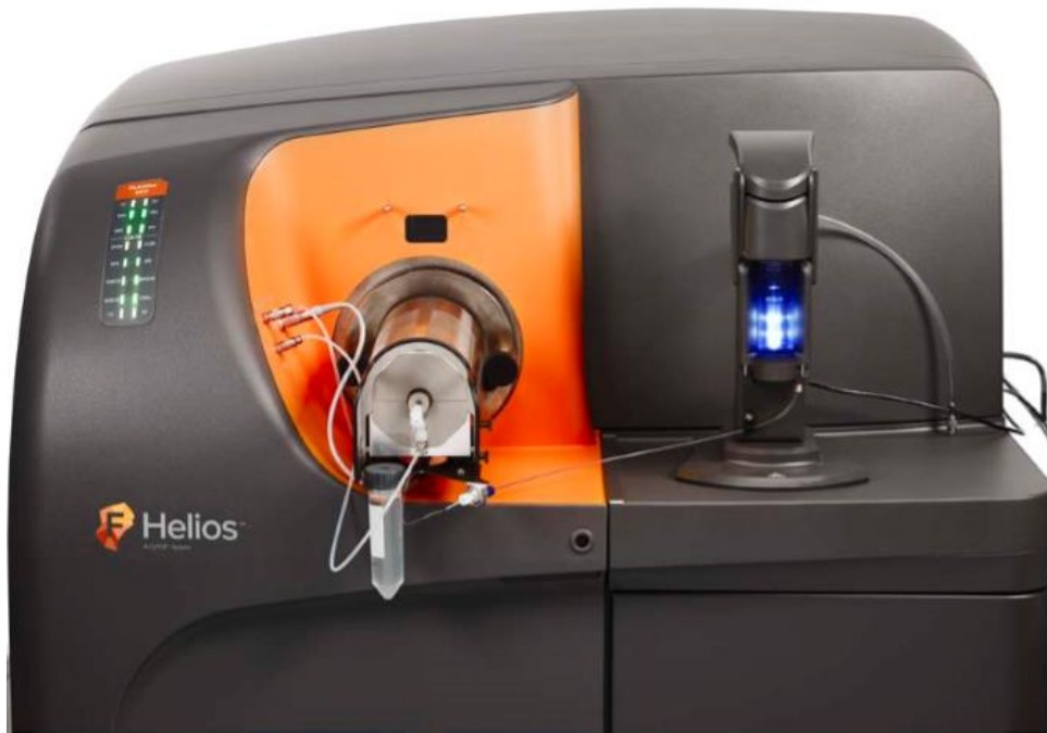
Figure 2.2: Fluidigm's mass cytometer model Helios. The Helios differs from other mass cytometer systems by having the autosampler instead of a syringe pump to inject the sample. The autosampler can be seen standing on the shelf on the right side of the machine. Reproduced from [44].
