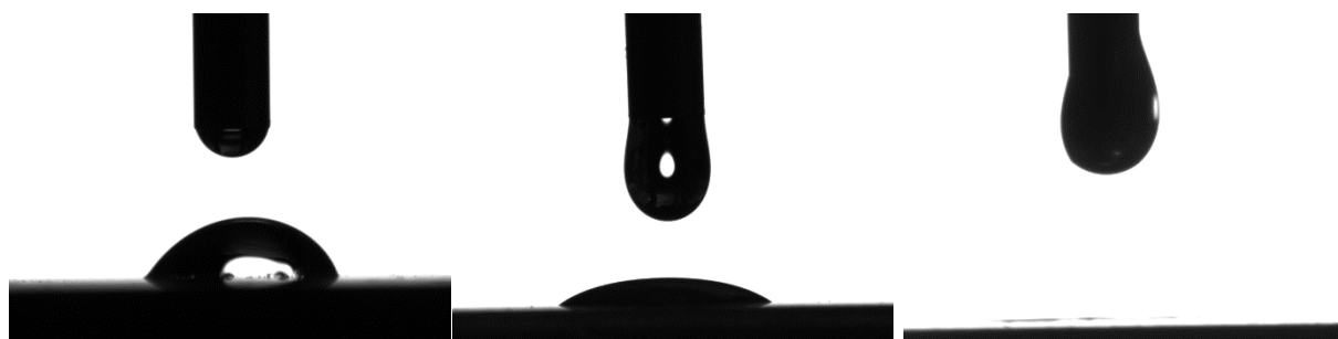
Figure 5.66. Optical contact angle measurements show water, diiodomethane and hexadecane droplets, respectively, deposited on an aluminum slide etched in HCl for 10 minutes followed by immersion in \text{HNO}_3 + \text{CuSO}_4 for 6 minutes.
