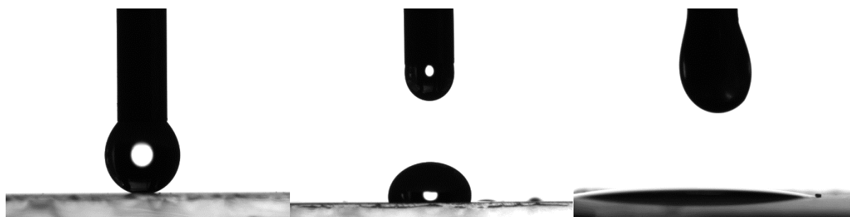
Figure 5.56. Optical contact angle measurements show water, diiodomethane and hexadecane droplets, respectively, deposited on a glass slide coated with soot from heating Oil DC 200.
