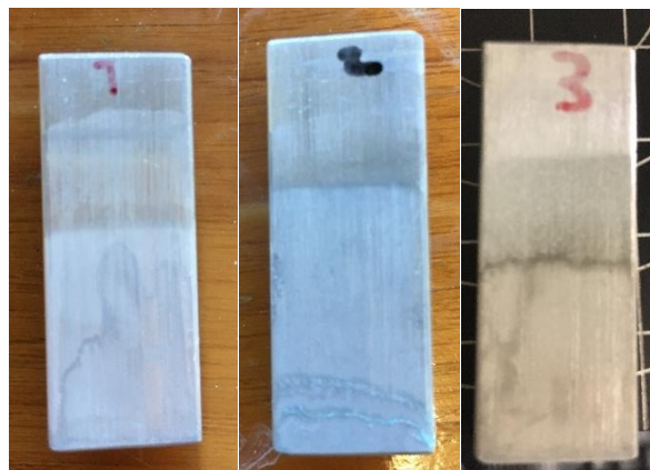
Figure A.12. Aluminum slide parallels one, two and three, respectively, etched 22 minutes in \text{HCl} and 6 minutes in \text{HNO}_3 + \text{CuSO}_4 , followed by coating in a solution of PDES and ethanol.
