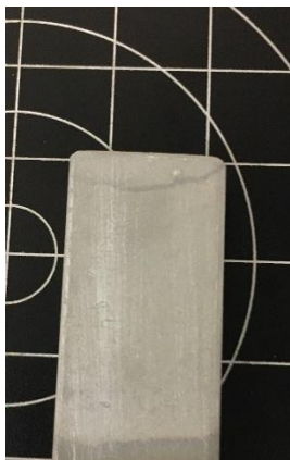
Figure A.11. Aluminum slide etched 10 minutes in and 6 minutes in \text{HNO}_3 + \text{CuSO}_4 followed by coating in a solution of PDES and ethanol.
