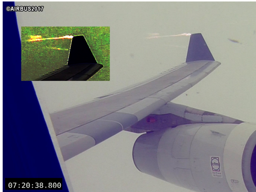
FIGURE 5.38: Camera observations of static discharge on the left wing during trigger 4.
