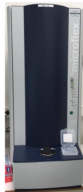
Figure 11. MALDI-TOF instrument used at VI for E. coli confirmation (Microflex, Maldi Biotyper)
