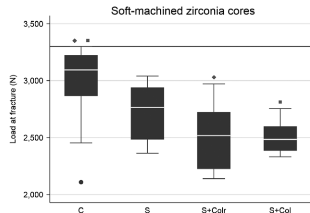
Fig. 6. Box plot of the four soft-machined groups with different margin designs. Further load was stopped at 3,300 N (horizontal reference line at y -axis) as a result of equipment limitation. The line within boxes represents the median, and the bottom and top of boxes represent the first and third quartiles, respectively. The maximum and minimum whiskers represent 1.5 interquartile ranges. Statistically significant differences between groups are marked with corresponding squares or diamonds. C, chamfer; S, slice; S + Colr, slice with cervical collar and reduced occlusal thickness; S + Col, slice with cervical collar.
