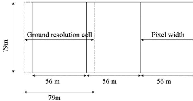
**Figure 6** The discrepancy between ground resolution and pixel size, modified from Lillesand and Kiefer (1994).
