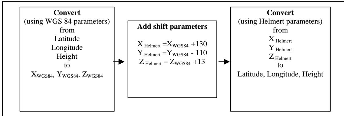
Figure 23 Three-parametric datum conversion of coordinates
