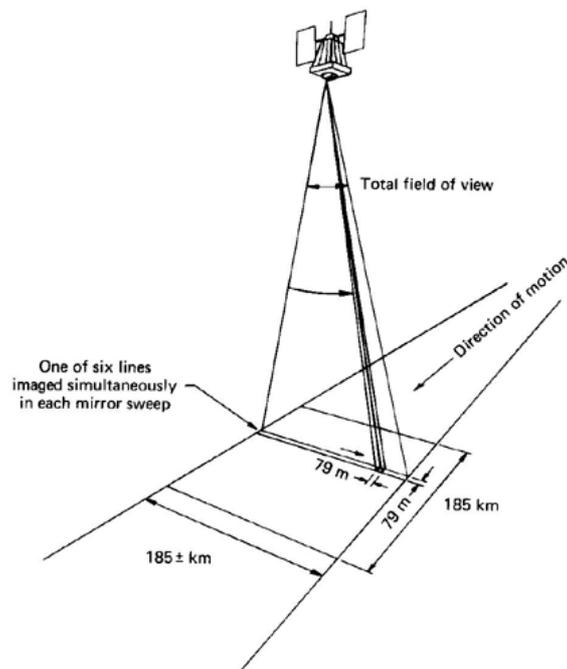
**Figure 5** The across tracking scanner exemplified by Landsat MSS, retrieved from Lillesand and Kiefer (1994).
