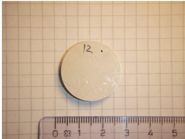
FIG 5.2. A photograph of one of the Pz27 disks (marked element no. 12) used in the prototype transducers, with diameter D = 24.888 mm and thickness T = 3.942 mm, resulting in a D/T = 6.31 .
