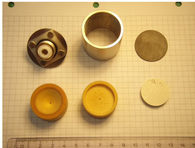
FIG 5.8. All mechanical parts of the piezoelectric transducer. Second row, from left to right: the casing plug, the casing and the front layer. First row, from left to right: the backing layer no. 2 (towards the back of the transducer), the backing layer no. 1 (towards the Pz27 disk) and the Pz27 disk.
