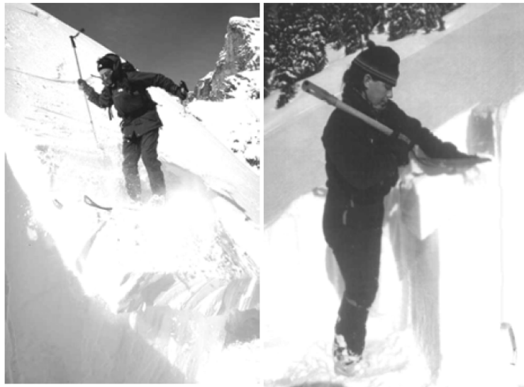
Figure 2.6 – Rutschblock test(left) and compression test (right), photo from: Schweizer and Jamieson (2004)
