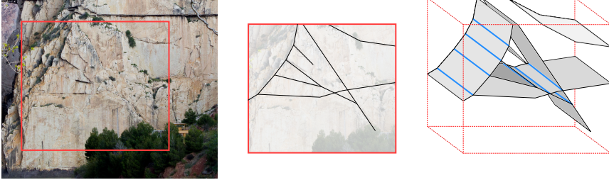
Figure 2.3: The left figure shows an outcrop of a fractured rock where the length scale of the fractures is tens of meters. The middle figure shows the dominant fractures traced by black lines. The right figure shows a conceptual model of an imagined 3d fractured porous medium. In the conceptual model the rock matrix is 3d, the fractures are 2d surfaces, and the intersections of the fractures are 1d (blue) lines.
