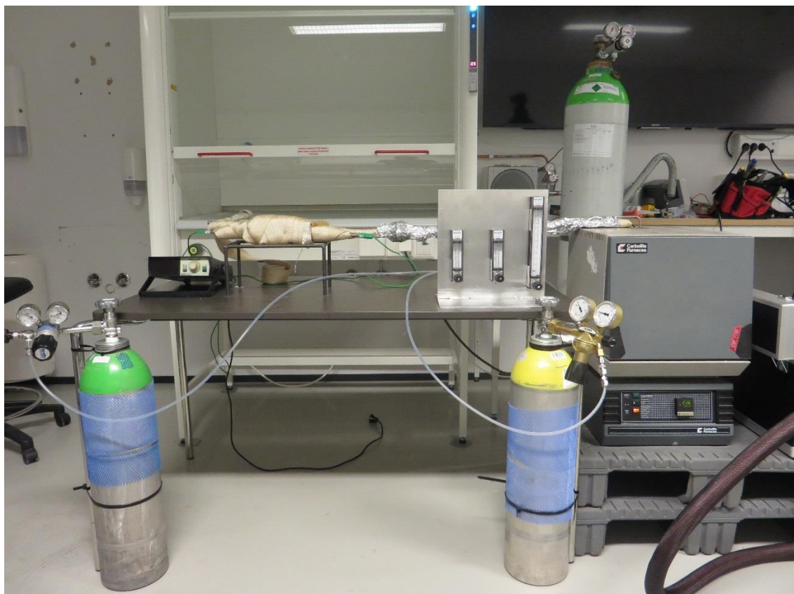
Figure 42 - Gas flasks connected to the SCR-system
