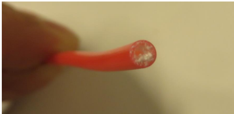
Figure 45 - Clogged intake tubes of HORIBA
