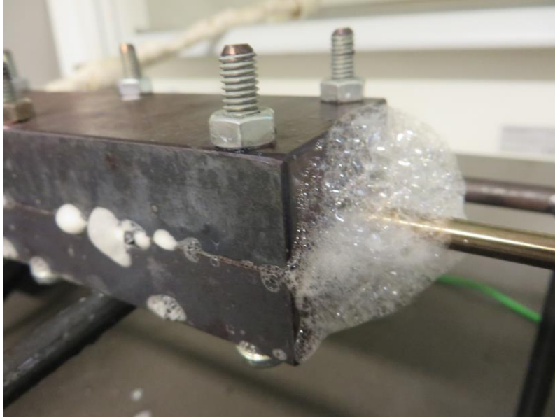
Figure 1 - SCR-reactor exposed for pressure of 2 bar
