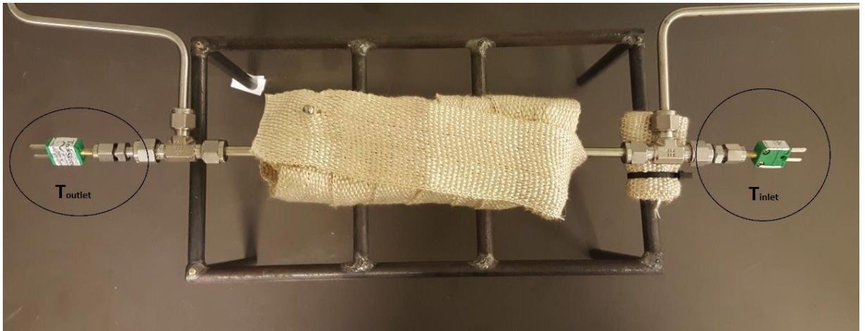
Figure 38 - Temperature sensors coupled at reactor inlet and outlet
