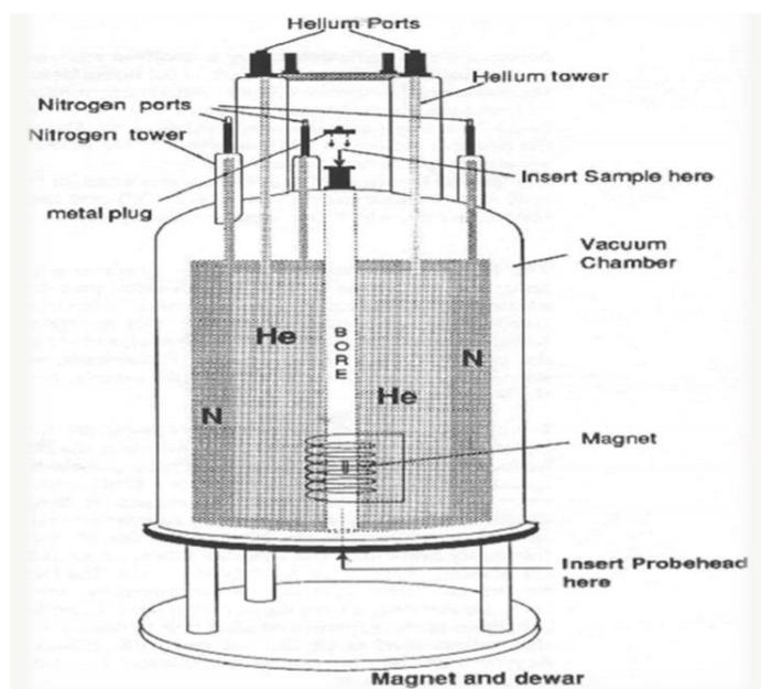
**Figure 6: The inside of a modern cryomagnet[13]**
