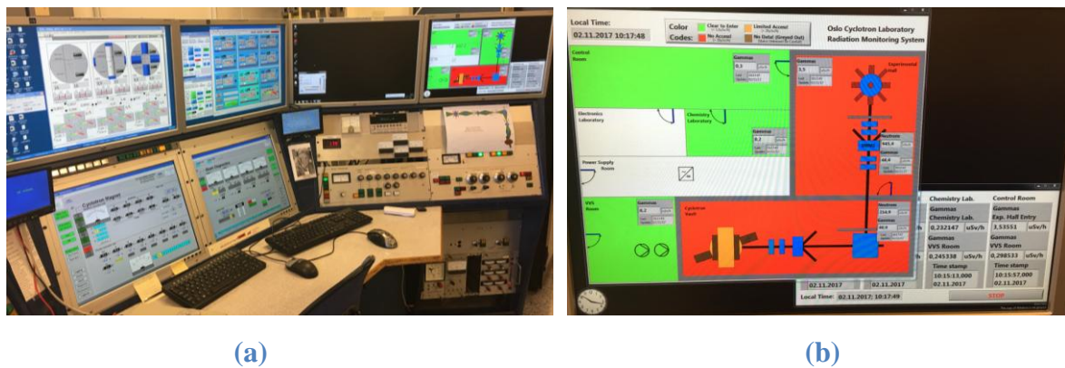
Figure 27: (a) Beam monitoring window (b) Measuring Gamma and Neutron incidence simultaneously.
