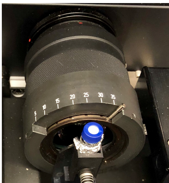
Figure 10. Illustration of how the samples were positioned for obtaining the Raman spectra. A piece of aluminum foil was placed and fixed behind of sample in the sample holder to avoid spreading of radiation.
