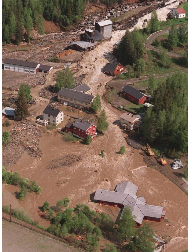
Figure 2.4: The flood in Tretten. The river Mokså diverted through the town, causing erosion of house foundations and sedimentation in the town. Photo: Eeg J. (1995)
