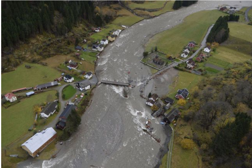
Figure 2.3: The flood in Flåm. There is considerable erosion on the banks of the river, endangering and destroying several houses. Photo: Mikalsen (2014)
