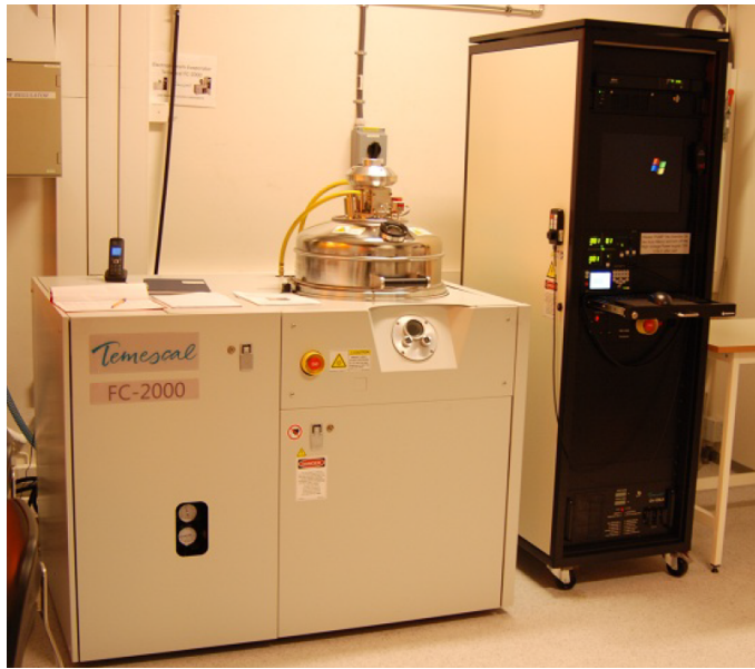
Figure 3.2: Picture of the Temescal FC-2000 situated in the semi-clean room at the UiB Nanostructures Laboratory. Picture from Bolstad (2012). 62
