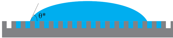
Figure 2.7: Schematic of a liquid droplet resting on a periodically rough surface with some of its volume propagating into the texture of the solid, a phenomenon called hemi-wicking.
