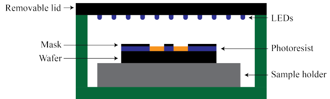
(b) Schematic of photolithography setup built in-house at the UiB NanoLab. Exposed resist is indicated with an orange color. Redrawn from Bolstad (2012). 62
