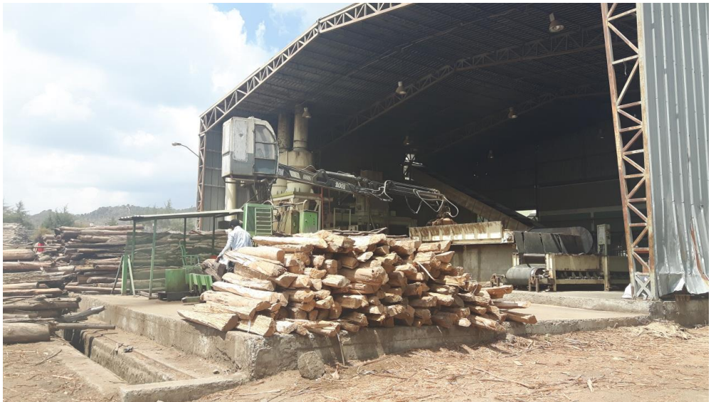
Fig. 2: Raw materials ready for chipping in particleboard manufacturing in Ethiopia (Photo: Akeza)
