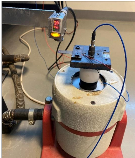
Figure 37: Close-up picture of piezoelectric cantilever harvester setup attached to a shaker
