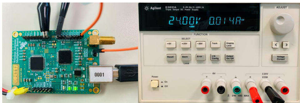
Figure 16: DC power supply to the board
