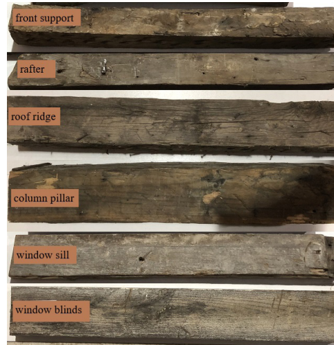
Figure 1: Macroscopic appearance of old wood materials from Zeytinlik houses.
