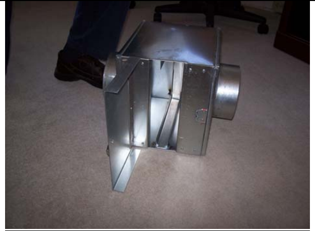
Figure 3-25 Custom designed outside air filter box installed in each house
