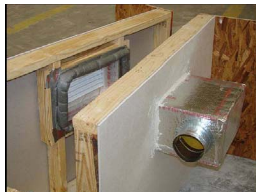
Figure I- 6 Southern Energy Homes Interior Crossover Duct Mockup
