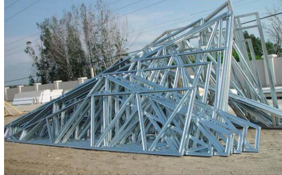
Figure 2- 24 Steel trusses produced on site
