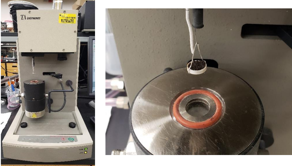
Figure 8: Thermogravimetric analysis (TGA) was used to monitor mass fluctuations of the pyrolants during ignition. The right image shows a sample of titanium and boron pyrolant mixture hanging on the weighing pan.
