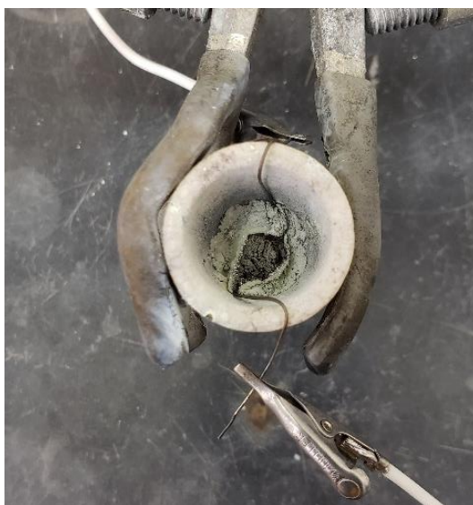
Figure 7: A post-combustion image of burned solid pyrolant in a ceramic crucible, atop a coiled nichrome wire. The reaction product has hardened around the wire coil.
