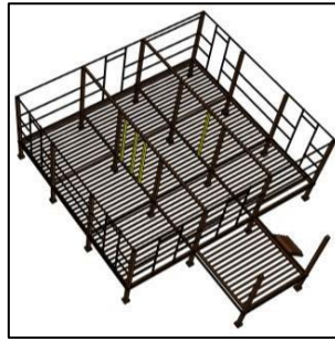
Figure 12 Main Column and support column
