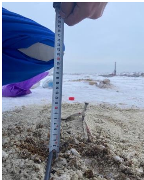
Figure 7. Measuring the thawed depth first day
