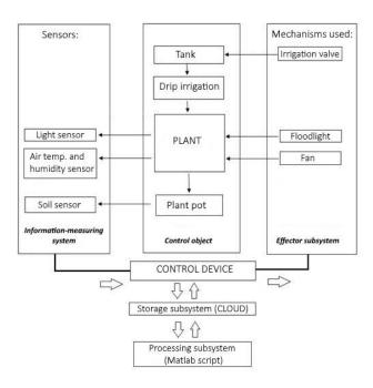
Figure 4. Functional diagram of an intelligent system
