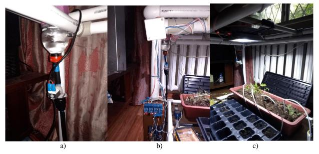
Figure 9. Home mini-greenhouse: a) irrigation valve; b) control unit; c) plants in the greenhouse
