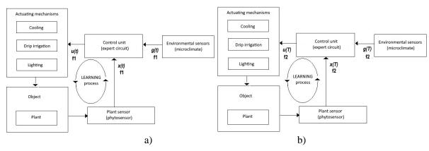
Figure 3. Control unit and data processing: a) in usage mode (f1); b) in training mode (f2)
