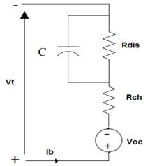
Figure 3. Simplifying model of battery
