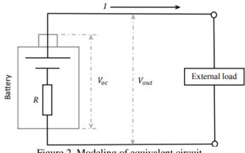
Figure 2. Modeling of equivalent circuit
