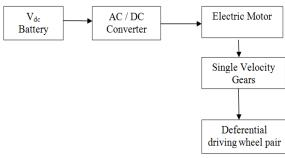
Figure 1. Battery electric Car power train scheme
