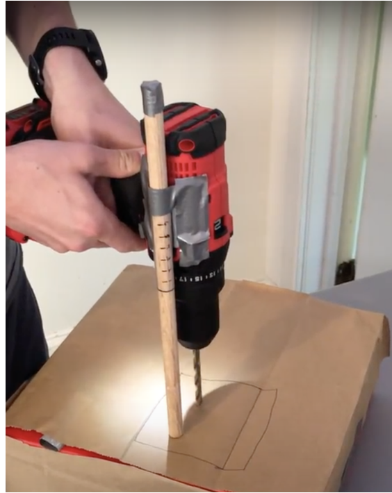
Figure 5. Final prototype for the depth measurement system. Measurements are in centimeters.
