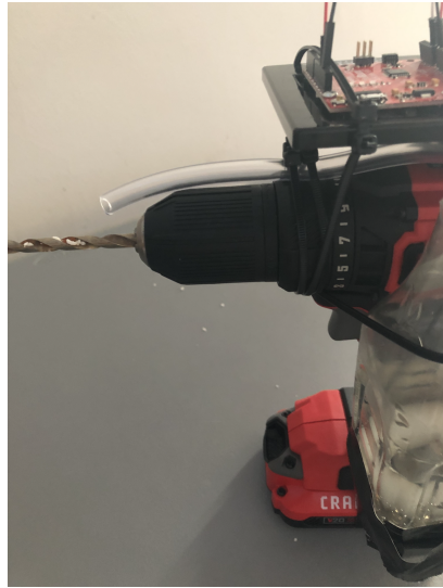
Figure 10. Image depicting the positioning of the tubing with respect to the drill and the bit.
