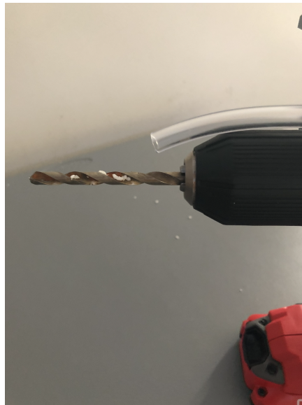
Figure 9. Image depicting the angled tubing that evenly dispenses the coolant over the drill bit.
