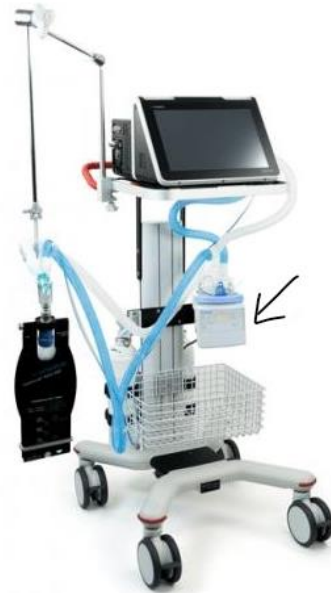
Figure 18. Bellavista 1000 ventilator showing the location of the humidifier machine (arrow pointing at it), connected but not incorporated in the ventilator [35].
