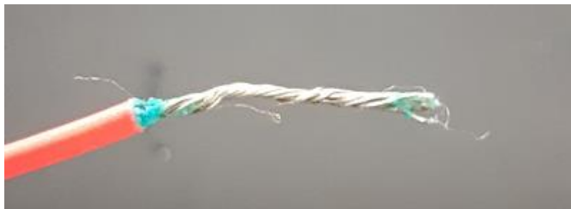
Figure 4 – Wire Oxidation Source: Authors
