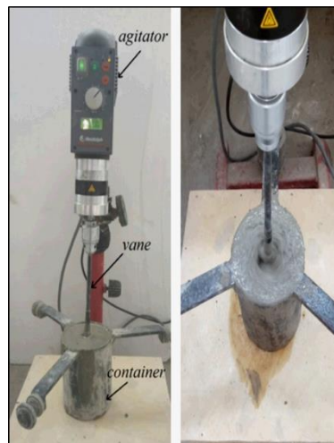
Fig. 8–The components of the rheometer.
