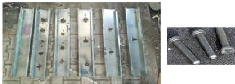
Fig. 2 - Galvanized Iron Channel section with stud connector.
