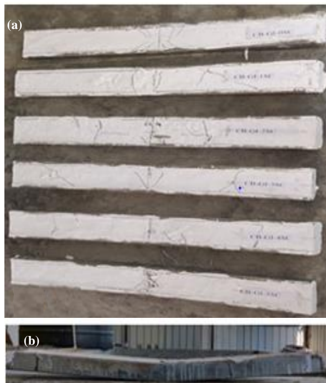
Fig. 9 – Composite beam after testing.
