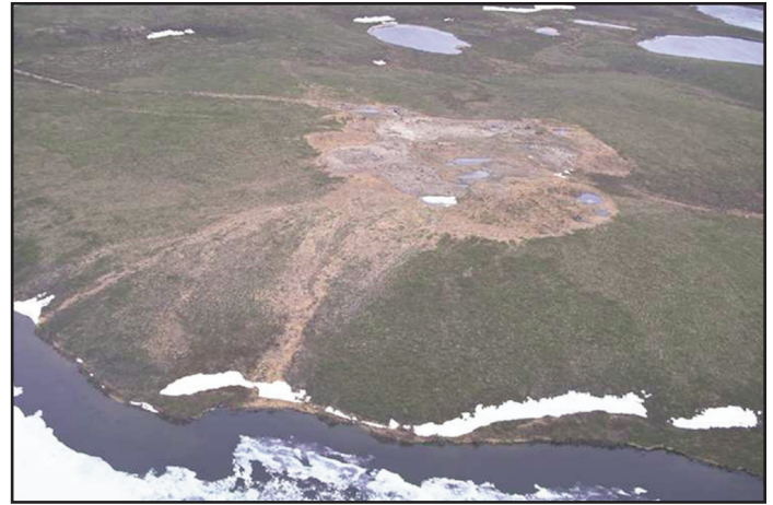
Figure 15. Failed drilling waste disposal sump at Parsons Lake, Tuktoyaktuk Coastlands, Northwest Territories, June 2004. Photo copyright © C.R. Burn.
