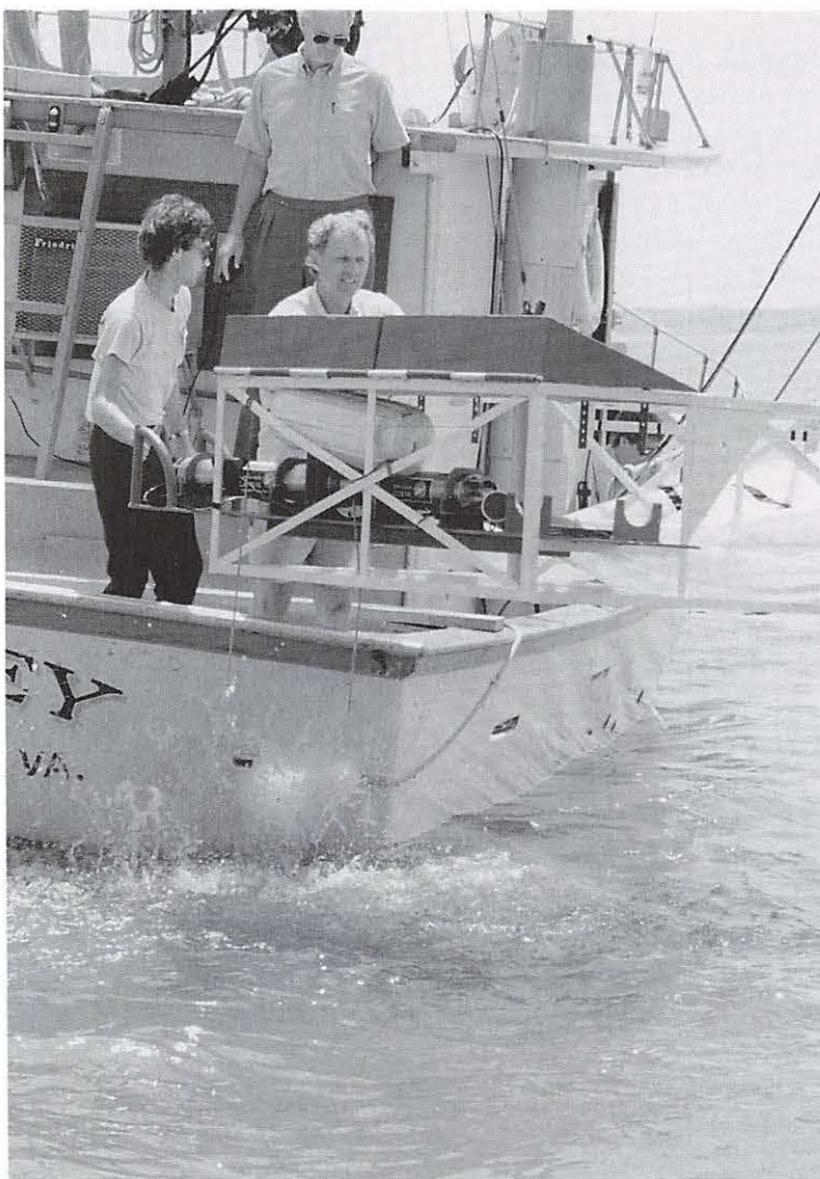
The plankton camera, developed and engineered by scientists in the Department of Biological Sciences, enables researchers to photograph marine organisms at the same time specimens are collected. A CTD device records salinity, temperature, and depth simultaneously with each photograph.
