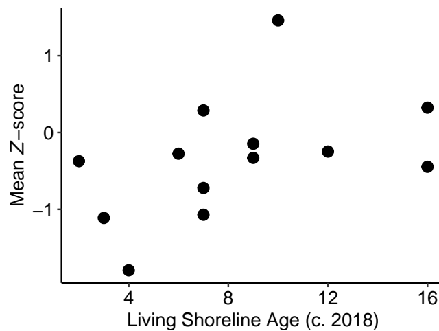
Figure 4 Net functional equivalence score vs living shoreline age. There was no detectable effect of the time since living shoreline construction on the net functional equivalence score across the 13 pairs.
