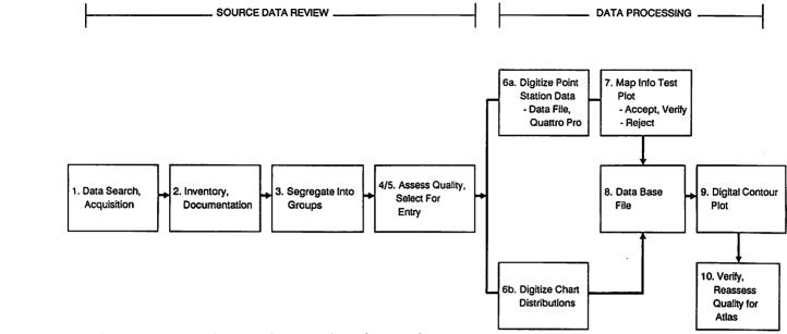
Figure 2. Scheme of organization and processing data into a computer data base and desk-top atlas.
