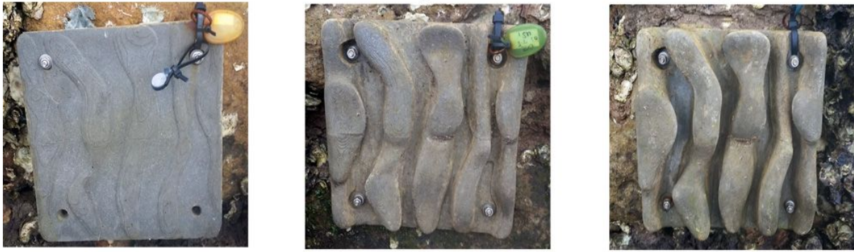
Fig 2: The three experimental treatments: a) flat, b) 2.5 cm complex, c) 5 cm complex.
