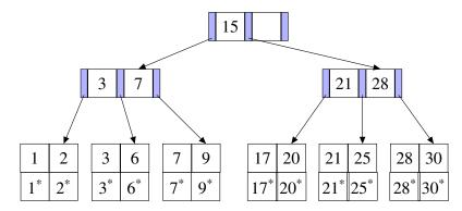
**Figure 3.2**: A 3-order B+ tree, where key-value pairs are stored only in leaf nodes (i.e., last level).
