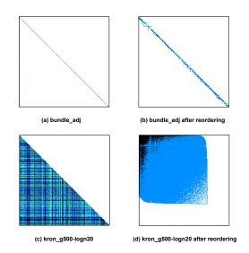
Figure 5.10: Visualization comparison of matrices with and without reordering
