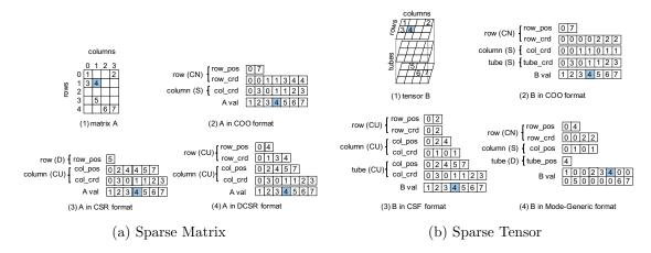
Figure 5.3: Example matrix and tensor represented in different formats. Each format is a combination of the storage format attributes.
