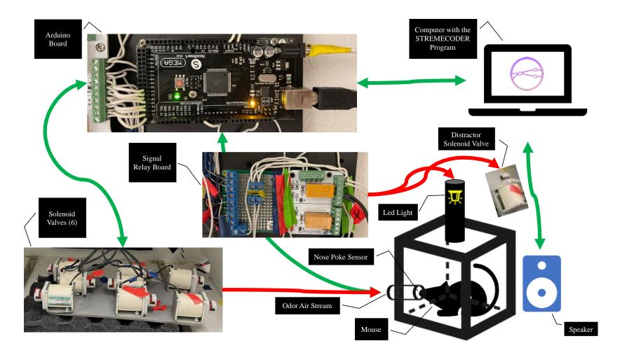
This schematic demonstrates how the rodent odor discrimination apparatus was set up. The green arrows represent from where the input and output are being sent and received, while the red arrows represent only where the output is being sent. This apparatus schematic only shows the necessary components needed to develop the program, there are more elements to the apparatus which are not displayed here.
