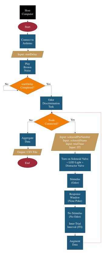
Flow chart illustrating the flow of information into and out of the STREMECODE program. The host computer initiates the start node which initiates various processes until the odor discrimination task is started. Once the task is started, it will traverse through all the nodes in an orderly looped fashion. When the traversal is completed, all data from the nodes will be aggregated and will be outputted as a CSV file.
