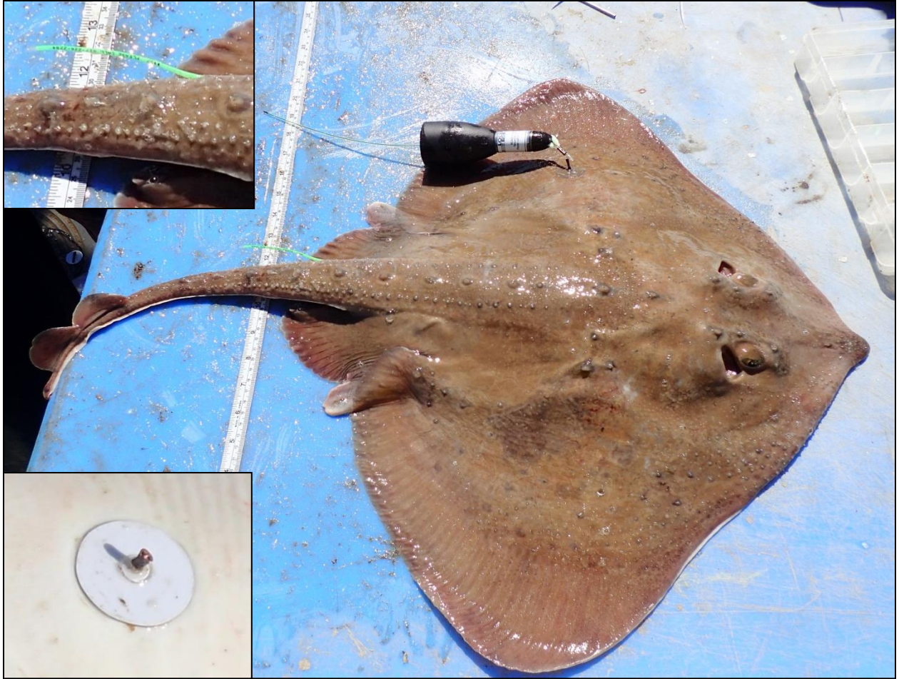
Figure 1.2. Pop-up satellite archival transmitting tag attachment method. Tags (Lotek LIFE LAT3500) were attached using monofilament line and two pairs of 1" Petersen discs and baffles secured on either side of the skate (dorsal and ventral). Image in the lower-left corner displays the Petersen disc/baffle/crimp pair on the ventral side of the skate. Image on the top-left corner displays the Floy® dart tag that was inserted at the base of the tail for all skates \geq 30 cm total length.
