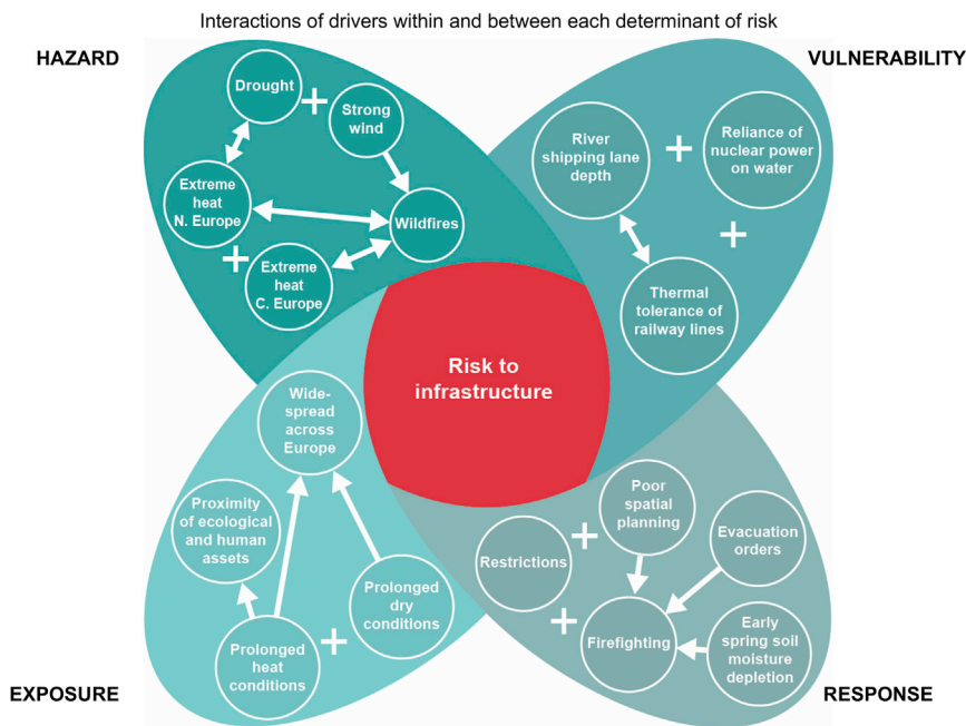
Figure 4. Complex interactions that generated risk to infrastructure during the 2018 European heatwave Arrows indicate interactions and addition signs indicate aggregation of the individual drivers of risk.
