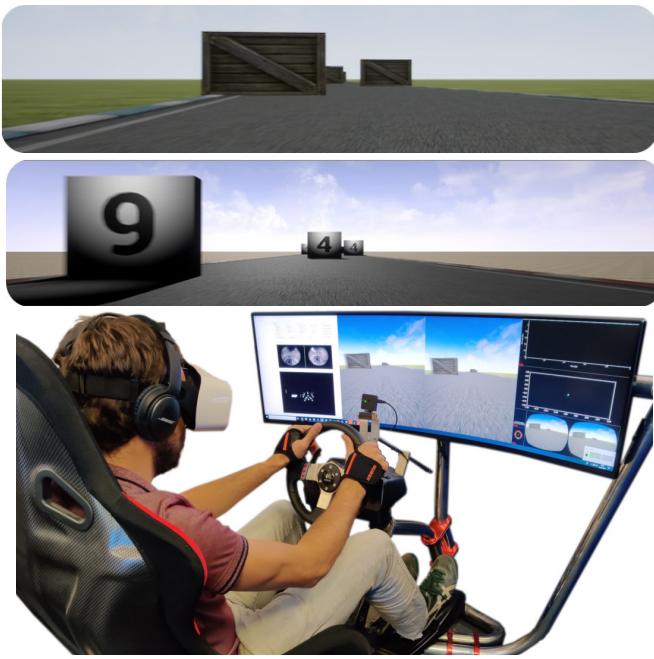
Fig. 3. Driver-in-the-loop simulation. Top: The two simulated scenarios. For the audio stimuli scenario, obstacles are simple boxes, while in the visual stimuli case, numbers are displayed directly on the obstacles. Bottom: The participant wears a VR headset with integrated eye gaze tracker and head pose estimation. The screen displays the scene observed by the participant and sensor readings in real-time for monitoring during the trial.
