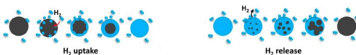
Figure 4.5 The illustration of the hydrogen absorption/desorption process in the metal particle. Adapted from [19] .
