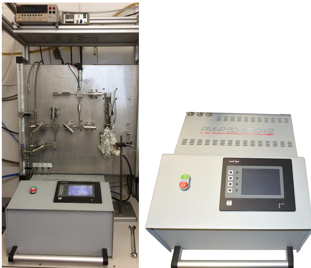
Figure A.5 Homemade Sievert's apparatus and the high-pressure compressor up to 1000 bar.
