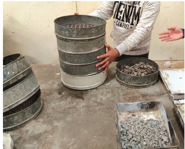
Fig. 2 — Sieve analysis being performed on coarse aggregate.
