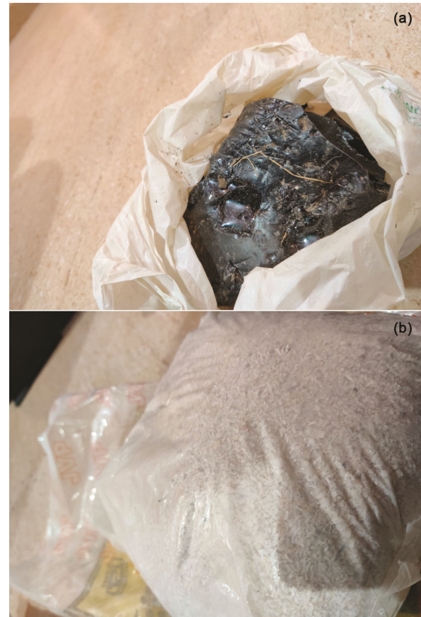
Fig. 1 — Raw materials for tests (a) VG 30 grade bitumen and (b) Marble dust.
