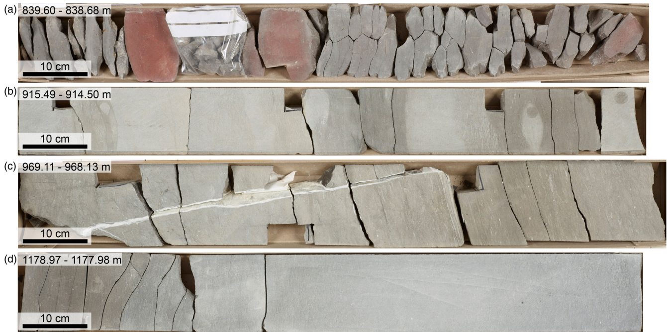
Fig. 4. Photographs of archive core sections with the section tops facing to the left. (a) Occurrence of siderite nodules in the lower Toarcian. Elevated Fe levels are visible as red surface staining of the aged archive core. (b) Calcite nodules in the upper Pliensbachian. Light, c. 8 cm-sized nodules are visible in the middle and lower parts of the core section. (c) Centimetre thick calcite veins in the upper Pliensbachian. (d) Typical dark–pale alternation on a metre scale in the lower Pliensbachian.
